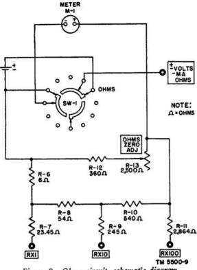
Figure 9. Ohms circuit, schematic diagram.
