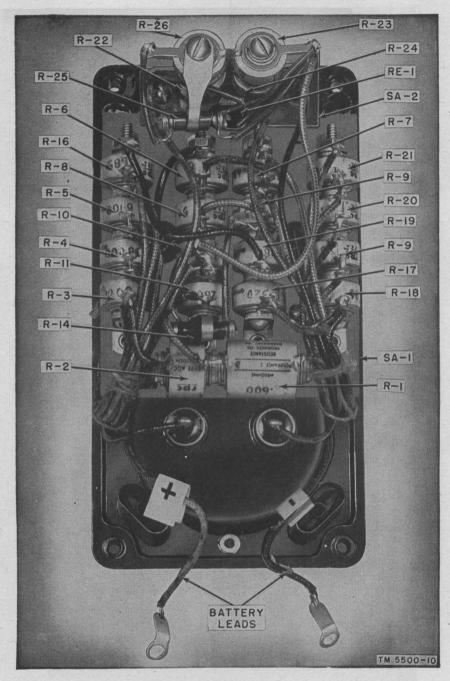
Figure 10. Multimeter subpanel.
