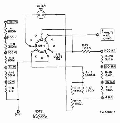
Figure 7. D-c volts-ma circuit, schematic diagram.
