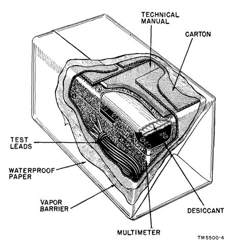
Fig. 4. Multimeter TS-297/U, cutaway view showing packaging details.
