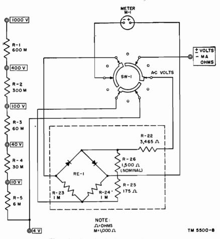
Figure 8. A-c volts circuit, schematic diagram.
