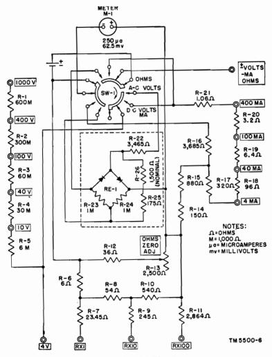
Figure 6. Multimeter TS-297/U, schematic diagram.
