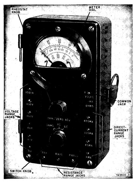
Figure 3. Multimeter, view of panel face.
