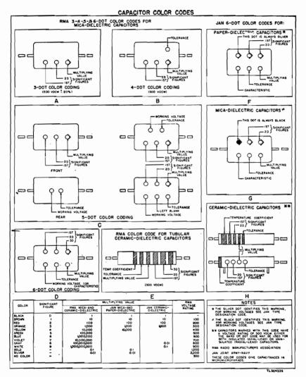
Figure 13. Capacitor color codes.
