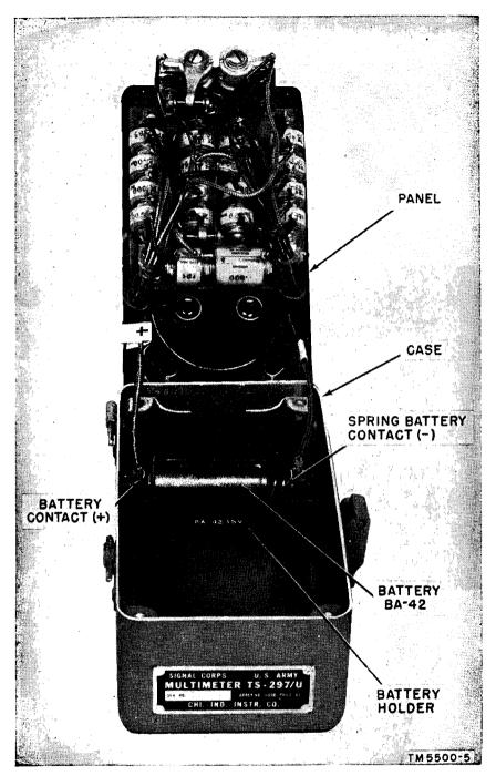
Figure 5. Multimeter, panel raised for installation of battery.
