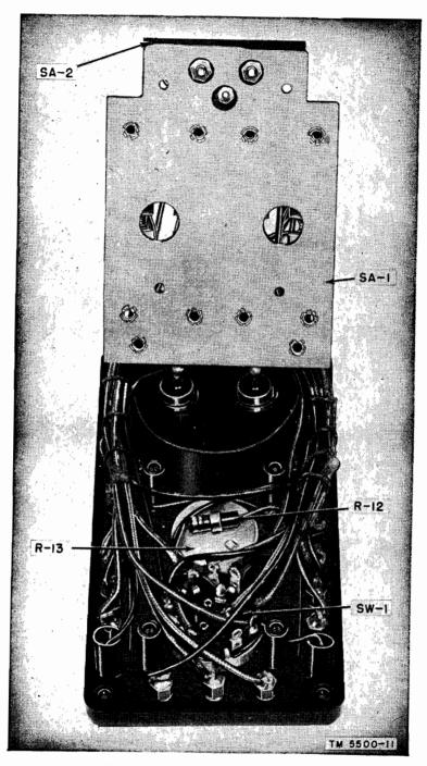
Figure 11. Multimeter, subpanel raised.
